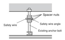
6. Connect the mounting base to the tip of the safety wire.
