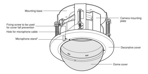
\* If a microphone is used, mount the microphone on the rubber-made microphone stand. Unless the microphone is used, cut the rubber with a nipper or conduct another treatment.
