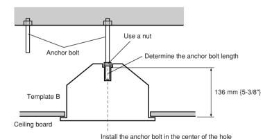
**Note:** If there is already an anchor bolt installed, the anchor bolt can be used as a second anchor bolt. Make sure that the distance between the 1st and 2nd anchor bolts is 1 000 mm {39-3/8"} or less before use.
